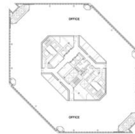
Floor plans of office spaces (The lower floors with squared layouts and the higher floors with hexagonal ones).
